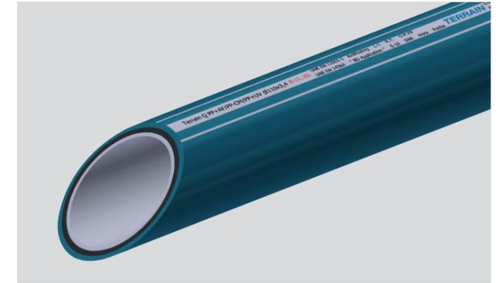
Terrain Q's multi-layered construction provides UV, impact and fire resistance. Its mineral-reinforced plastic delivers high-stability and noise insulation performance, whilst its inner layer is abrasion resistant, can withstand extreme temperatures from minus twenty degrees centigrade right up to ninety-five degrees centigrade, and has an anti-fouling additive for anti-encrustation protection.
