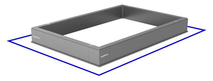
Mark a line around chamber for excavation footprint.
