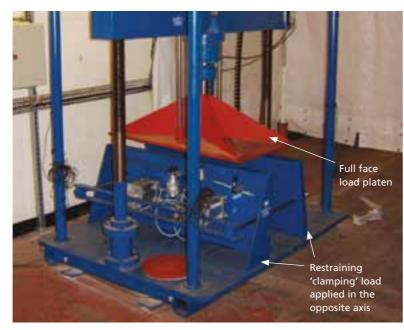
Figure 8 Compression test rig
