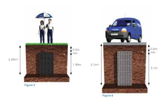
Note: \* Based on ground conditions being dense sand and gravel.
