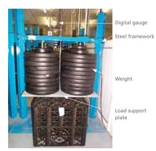
Figure 11 Creep test rig
